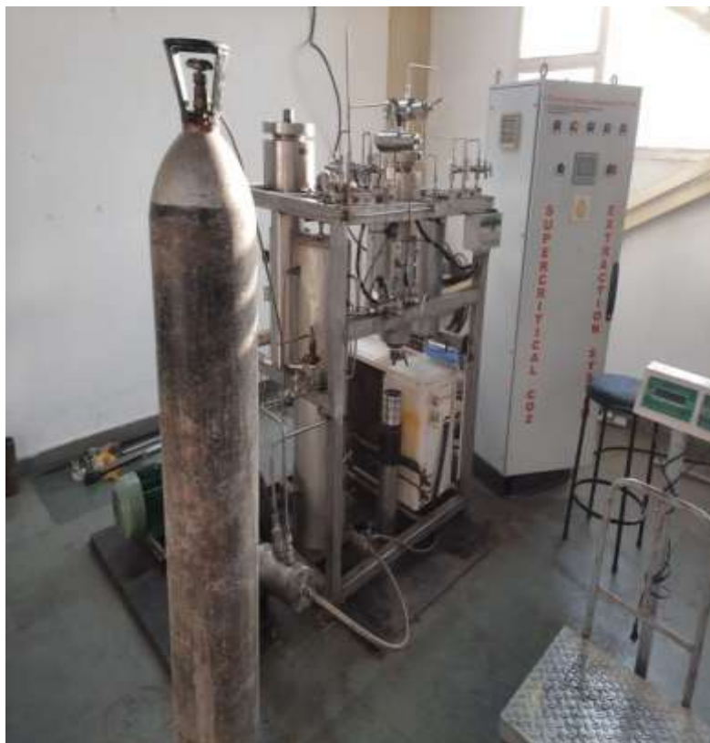
Fig-1 CO 2 Extraction Unit
