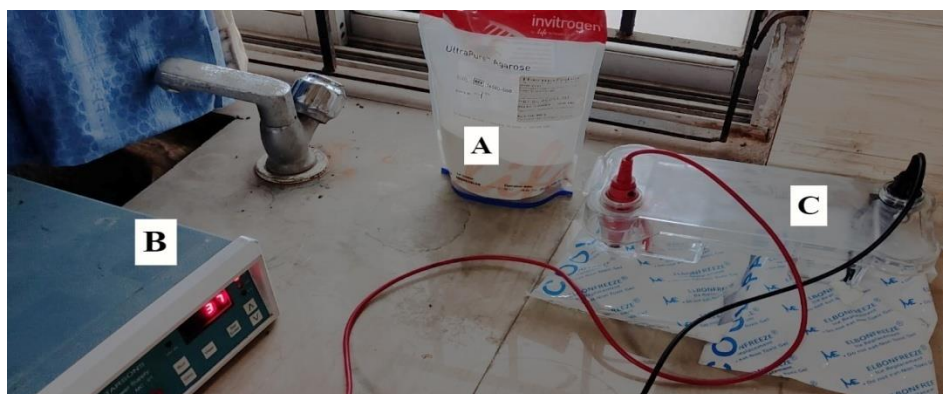
Fig 4: "A"-Agarose powder,"B"-power pack for electrophoresis,"C"-electrophoresis instrument kept on ice pack and connected to the power pack during the procedure
