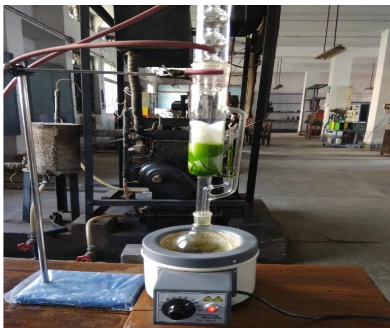
Fig.3 Soxhlet Extraction Process
