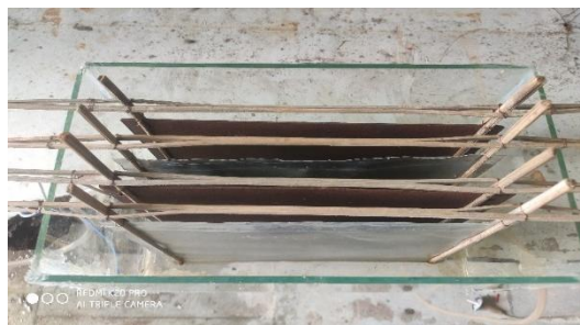
Fig.1. Figure showing basic skeletal frame of the reactor including aluminum and iron sheets as electrodes
