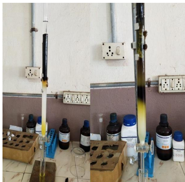
Figure-2: Column chromatography
