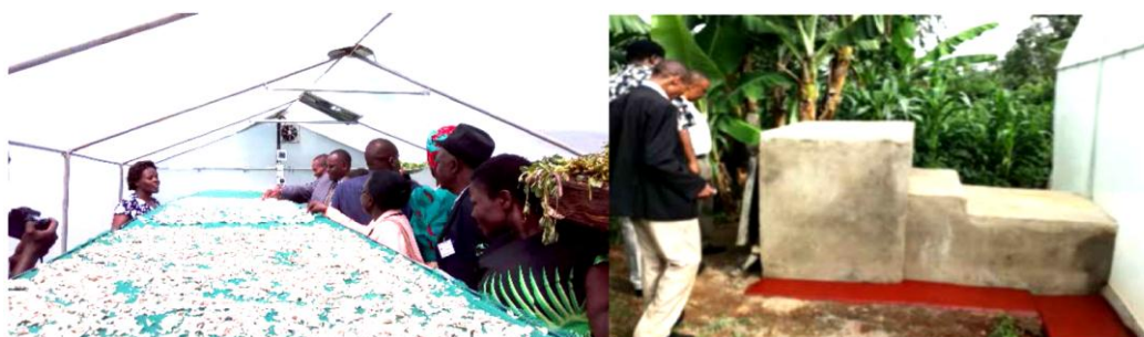
Figure 4. Left: Greenhouse Dryer. Right: The biomass heater for the hybrid dryer
