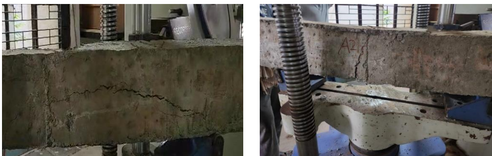
Fig. 4 Failure and cracking pattern of beams.
