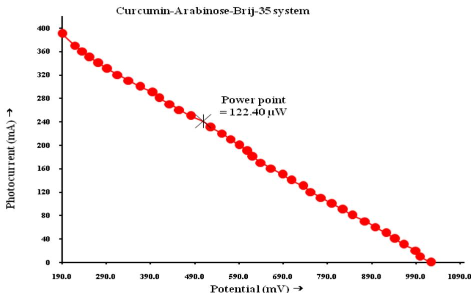
Fig. 3 CURRENT VOLTAGE (i-V) CURVE OF THE CELL.
