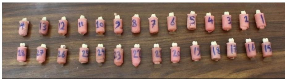
A picture showing the complete sample after the crowns have been cemented
