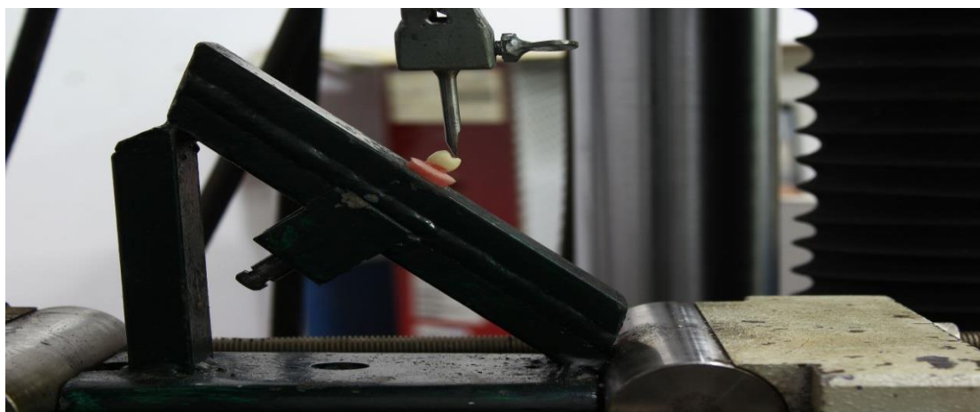
A picture illustrating the application of inclined forces at a 45-degree angle on a sample using the Universal Test Machine.
