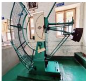
Figure 6: IZOD type of impact tester
