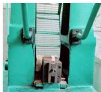
Figure 7: Sample placed in the metal fixture so that the middle of the sample coincides with the striking pendulum
