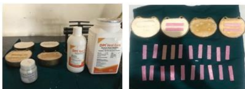
Figure 3b: Control specimen Non-reinforced PMMA
