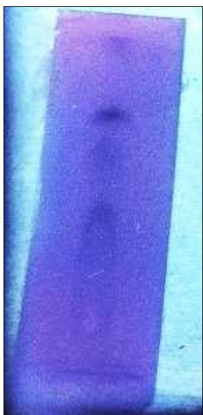
Fig 4 – Identification of boswellic acid -TLC plate under UV light chamber
