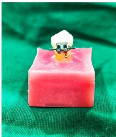
Figure 1. Test Unit with 5mm archwire ligated with ligature wire
