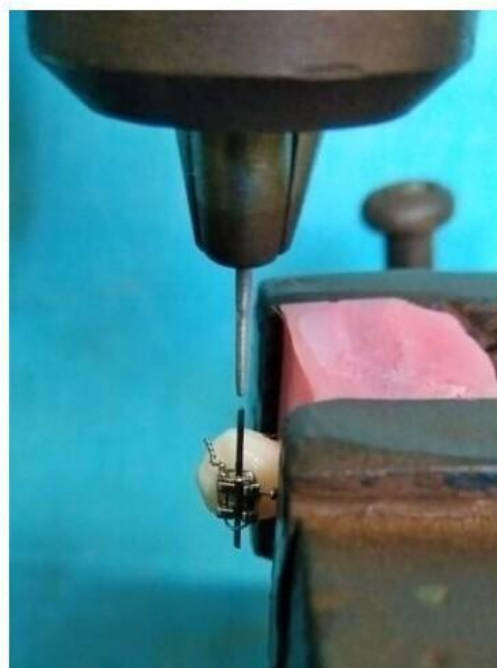
Figure 7. The wire was pulled, at a crosshead speed of 0.5mm/min; 25kN force.
