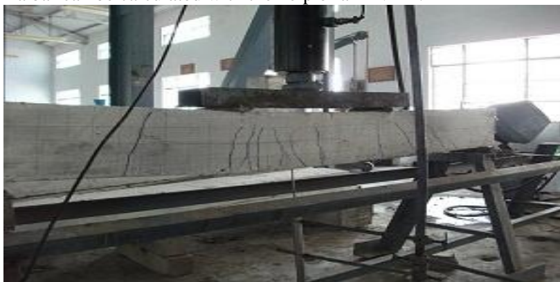
Figure 3. Setting for Flexural Strength Tests
