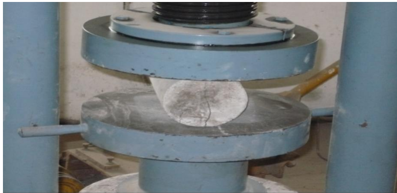
Figure 2. Setting for a Split Tensile Strength Test
