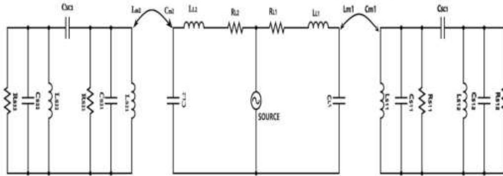
Figure 2: Equivalent circuit of the DFILA antenna with the VLSRR structures
