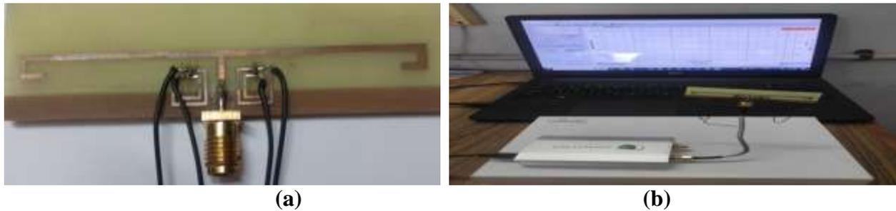
**Figure 3: Proto type model of DFILA with VLSRR Structure**
