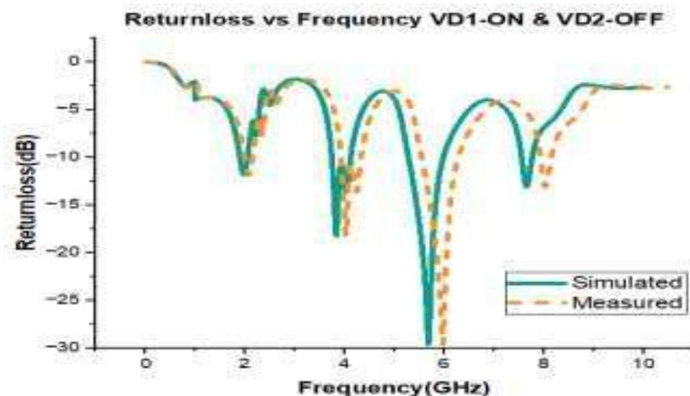
**Figure 6: Reflection Coefficient S11(dB) vs. Frequency(GHz) for switch case -3(ONOFF)**
