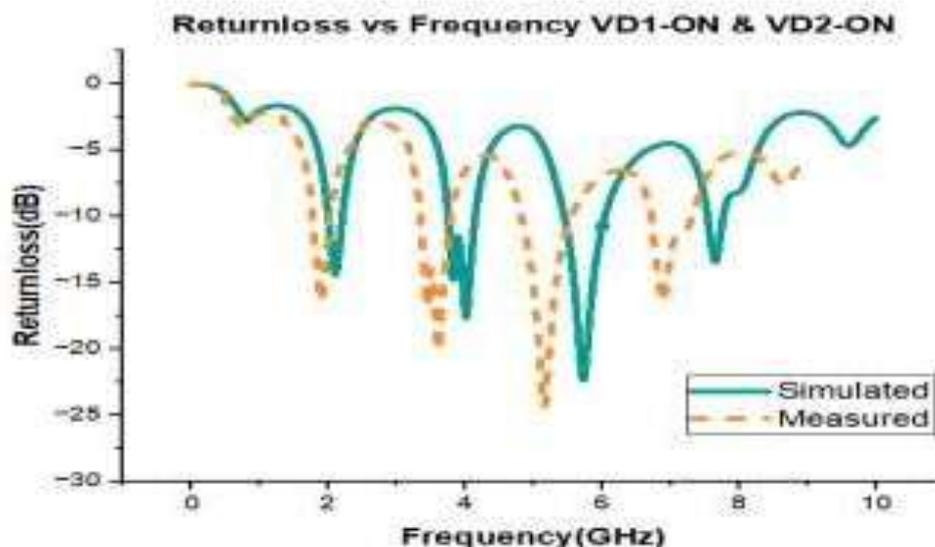
**Figure 7: Reflection Coefficient (S11(dB) vs. Frequency(GHz) for switch case -4(ONON)**
