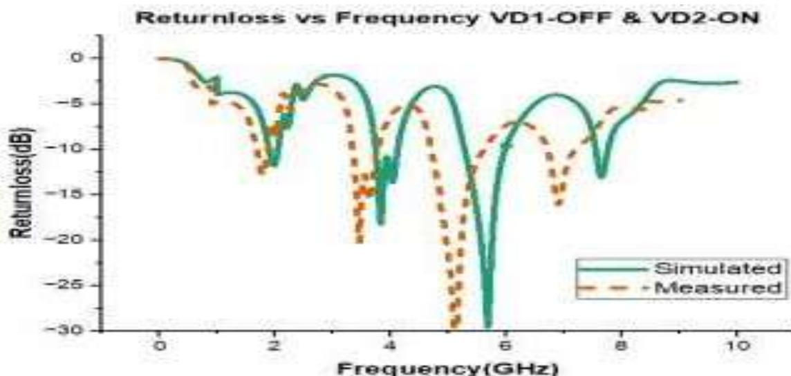
**Figure 5: Reflection Coefficient(S11(dB) vs Frequency(GHz) for switch case -2(OFFON)**
