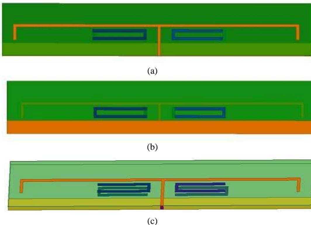
**Figure 1. Geometry of the Proposed Antenna (a)Front View (b)Backside View and (c)Top View**
