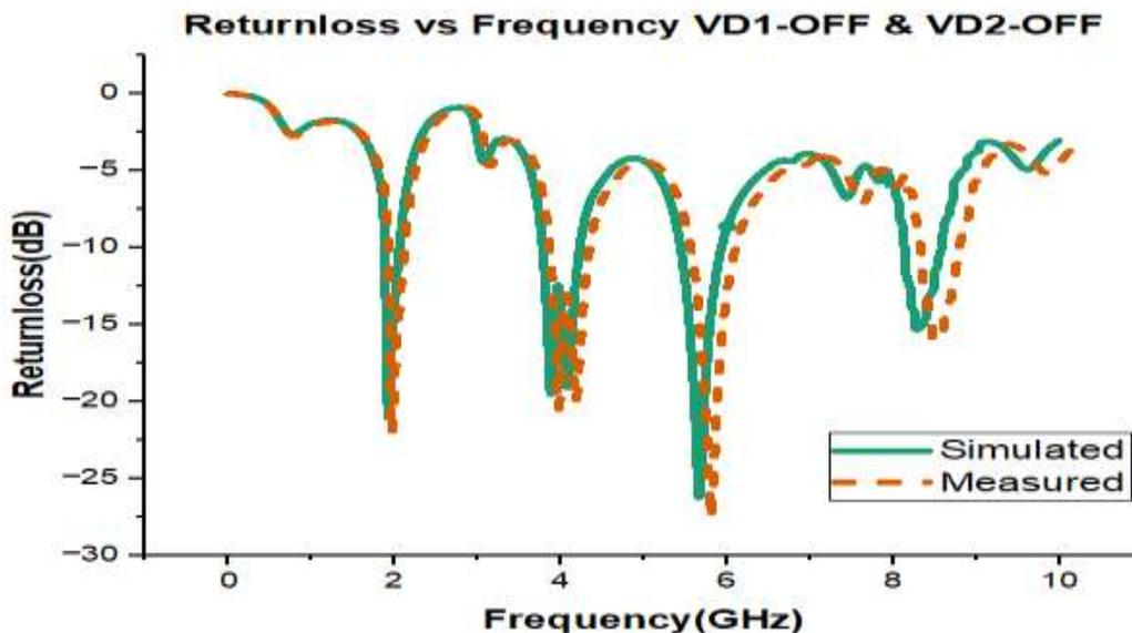
**Figure 4: Reflection Coefficient (S11 (dB) vs. Frequency (GHz) for switch case -1(OFFOFF)**
