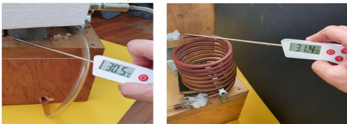
Figure 9- Examples of collection of data using food thermometer
