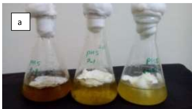
Figure 4.a- Pesticide degradation at pH5 (cypermethrin, Quinalphos, Control),b- Pesticide degradation at pH7 (cypermethrin, Quinalphos, Control) c- Pesticide degradation at pH9 (cypermethrin, Quinalphos, Control)
