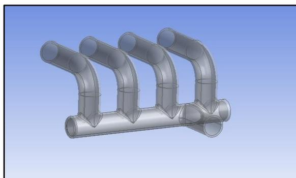
Figure 2: Design of exhaust manifold
