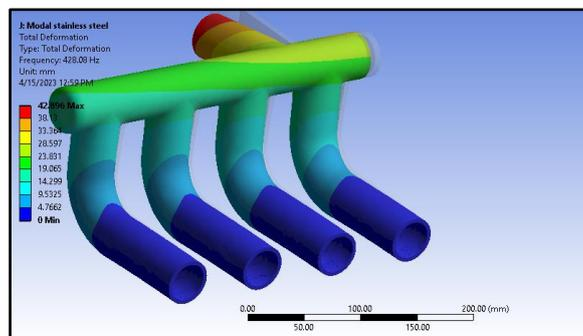
Figure 15: 1<sup>st</sup> mode shape of steel exhaust manifold
