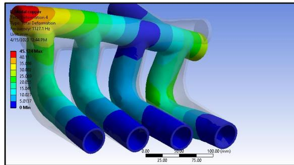
Figure 13: 4<sup>th</sup> mode shape of copper exhaust manifold
