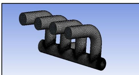
Figure 3: Meshed model of exhaust manifold
