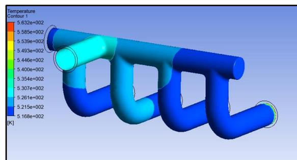
Figure 8: Temperature distribution plot on exhaust manifold
