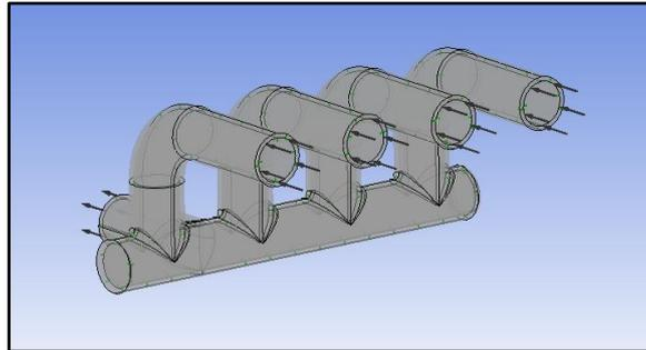
Figure 4: Loads and boundary conditions
