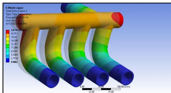
Figure 11: 2<sup>nd</sup> mode shape of copper exhaust manifold
