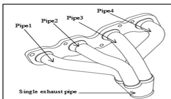
Figure 1: Schematic of the exhaust manifold of a four-cylinder naturally aspirated engine [1]
