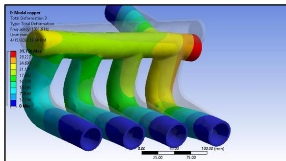
Figure 12: 3<sup>rd</sup> mode shape of copper exhaust manifold
