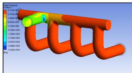
Figure 6: Total pressure distribution on exhaust manifold
