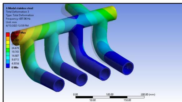
Figure 17: 3<sup>rd</sup> mode shape of steel exhaust manifold
