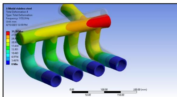
Figure 18: 4<sup>th</sup> mode shape of steel exhaust manifold
