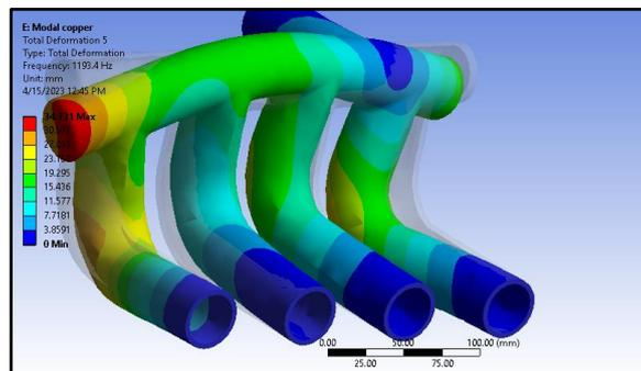
Figure 14: 5<sup>th</sup> mode shape of copper exhaust manifold
