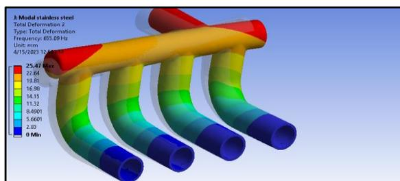
Figure 16: 2<sup>nd</sup> mode shape of steel exhaust manifold
