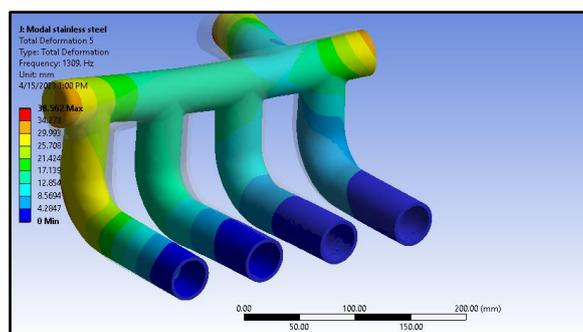
Figure 19: 5<sup>th</sup> mode shape of steel exhaust manifold
