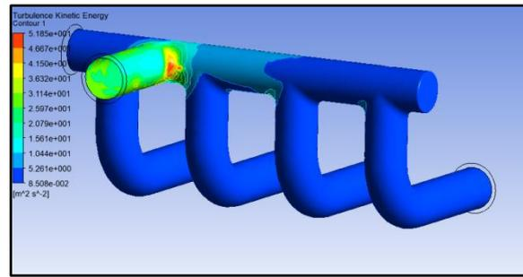
Figure 7: Turbulence kinetic energy distribution plot on exhaust manifold
