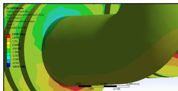
Figure 9: Heat flux plot on exhaust manifold
