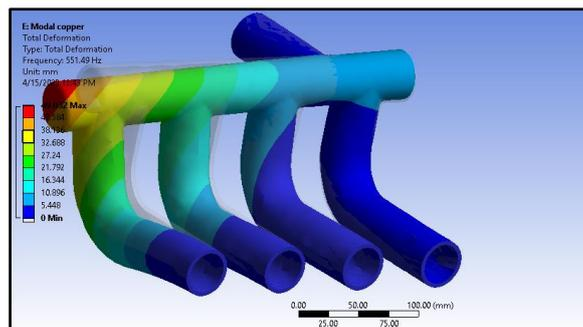
Figure 10: 1<sup>st</sup> mode shape of copper exhaust manifold
