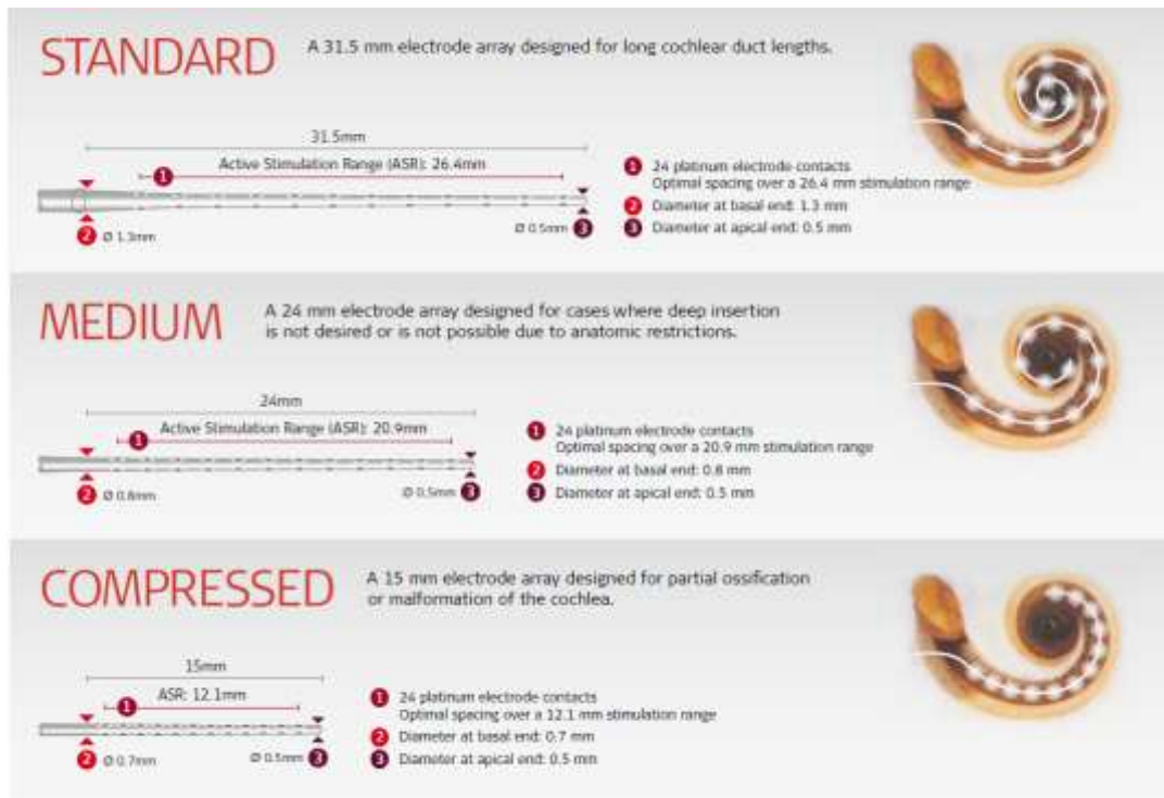
Fig-2 Classic series electrodes detailed description (courtesy of MEDEL Company)
