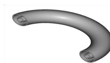
Fig7: Close-up of double pipe coil
