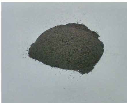
Figure 2- Bagasse ash used in the research
