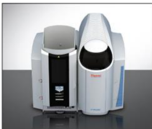
Figure 2: Model of Thermo Scientific iCE 3000 Series Atomic Absorption Spectrometer at USIC Department, Gulbarga University Kalaburgi Karnataka India.
