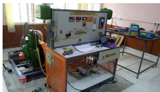
Fig. 2: Computerized Diesel Engine Test Rig
