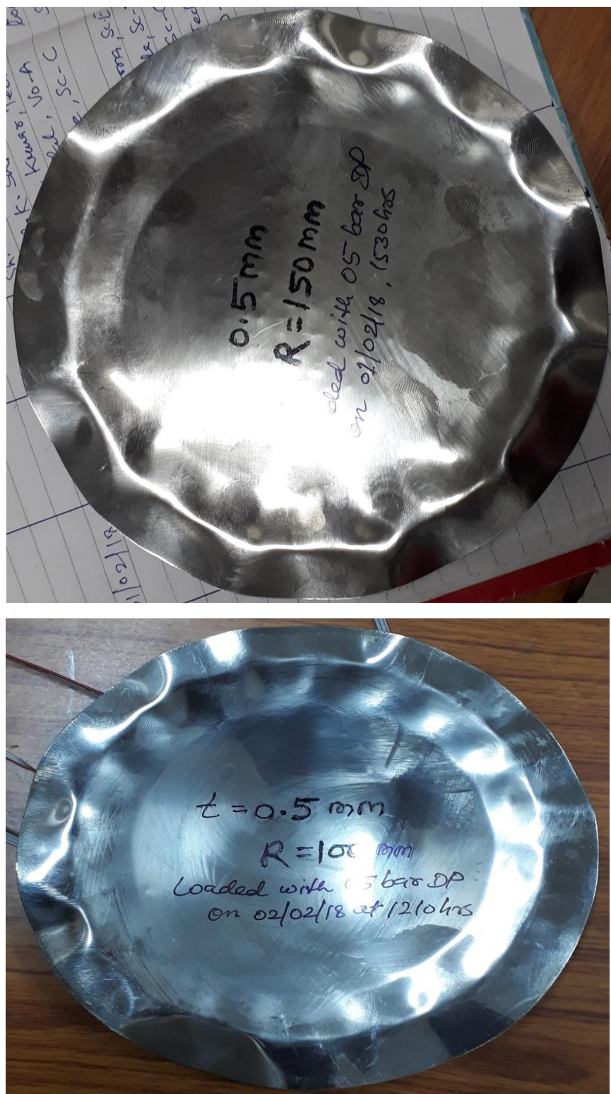
Figure 5.17: Photographs of plastically deformed 0.5 mm thick hemispherical shells
