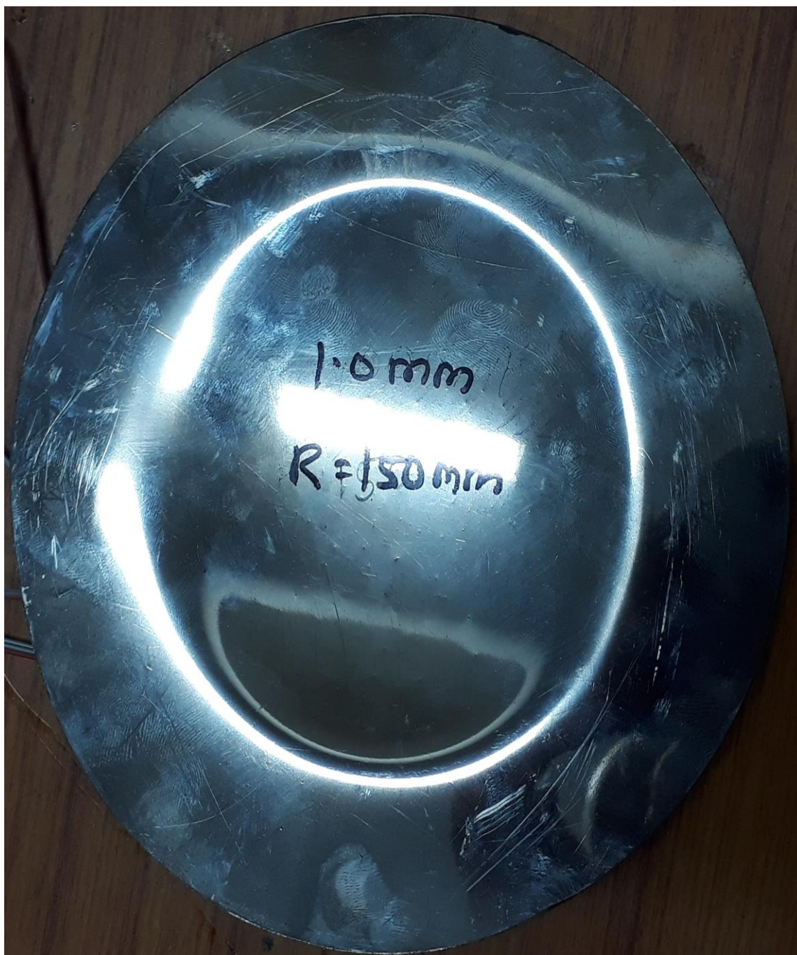
Figure 5.20: 1 mm thick shell with 150 mm radius of curvature
