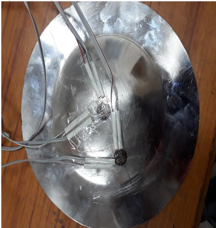
Figure 2.1: Hemispherical shell with 2r curvature and thickness 1.5 mm
