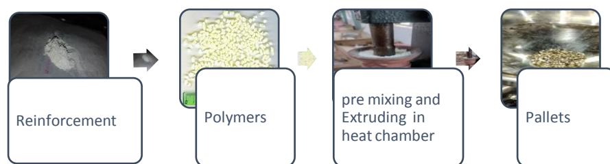
Fig.3.Sequence of steps of composite pellets manufacturing
