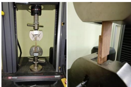
Figure 3: Tensile strength testing of sodium silicate adhesive on wood blocks
