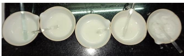
Figure 1: Prepared samples of modified sodium silicate with gum arabic (2% to 10%)
