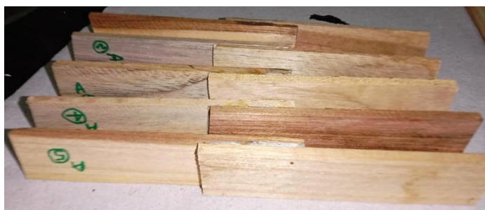
Figure 2: Preparation of wood blocks for water resistance investigation
