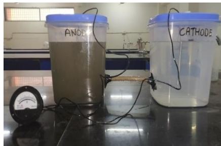
Fig 2: Experimental setup of Double chamber bacterial fuel cell
