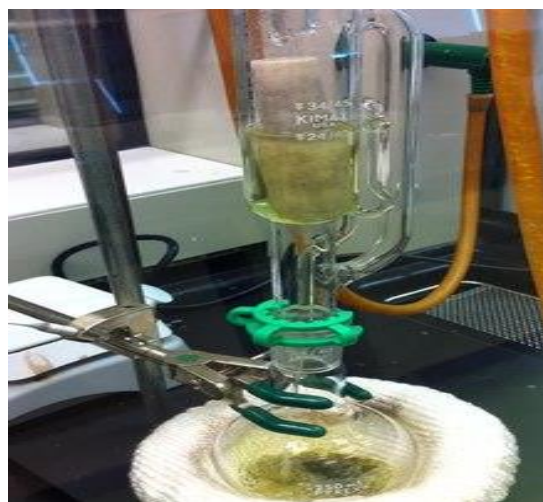
Figure 1: Soxhlet extraction of Plant Material
