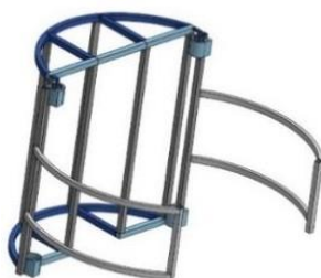
Figure 1 Model of Two-wheeler containment and charging apparatus
