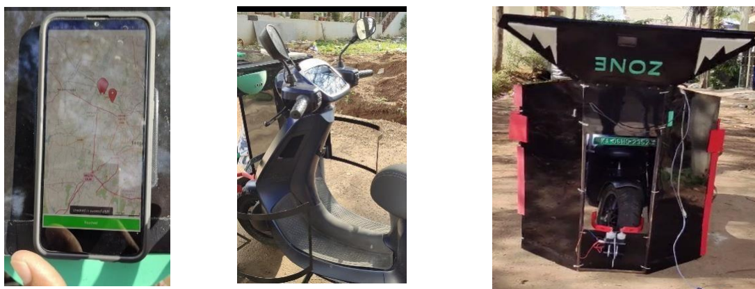
Figure 10(a)(b)(c) Check in successfully -message received and body and wheel lock actuated
