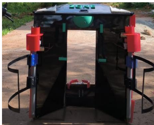
Figure 3 Working two-wheeler containment and parking apparatus prototype (unlock position)
