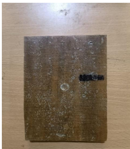
Figure 9: Specimen after Drop Weight Impact Test
