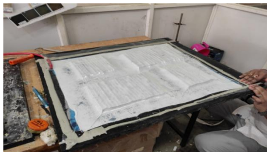
Figure 4: Vacuum Bagging Process
