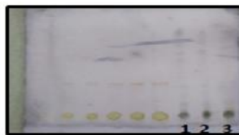
Fig 9 - HPTLC fingerprints of different brands of Rhus toxicodendron mother tinctures (samples 1,2 &3) after derivatisation
