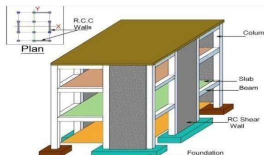
Fig 1.3 Shear walled frame system
