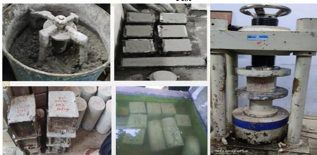
Fig. 1. Casting, curing and testing of concrete samples
