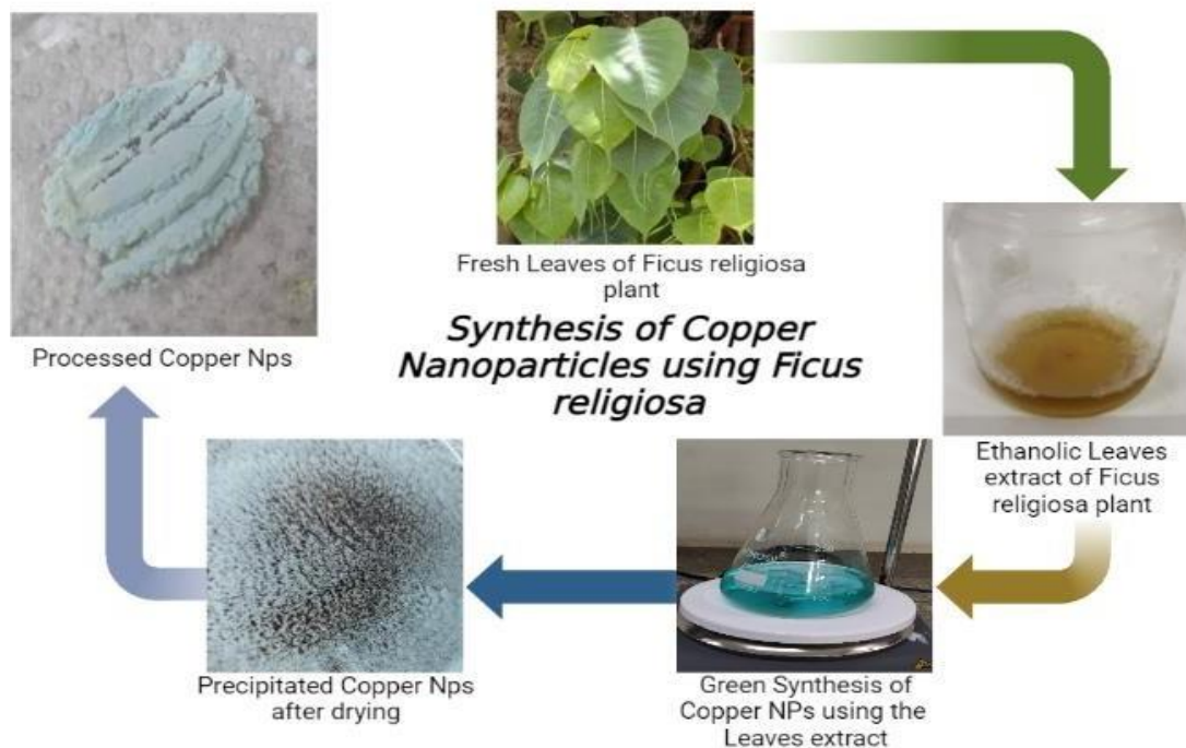
Figure 7 Shows the results of the Green synthesis of FCu NPs using Ficus religiosa leaves extract.
