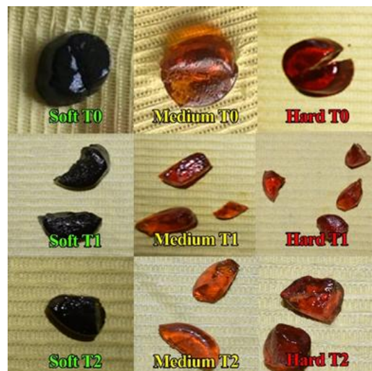
Figure (4): Pattern of chewing in 3D printed denture.
