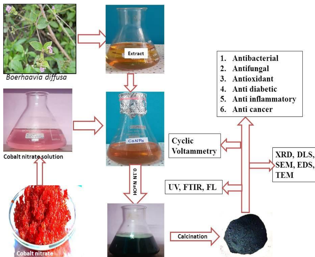
Figure:1 Scheme Green synthesis of cobalt oxide nanoparticles by Boerhavia diffusa , spectral characterization, Morphological, electrical and Pharmacological studies
