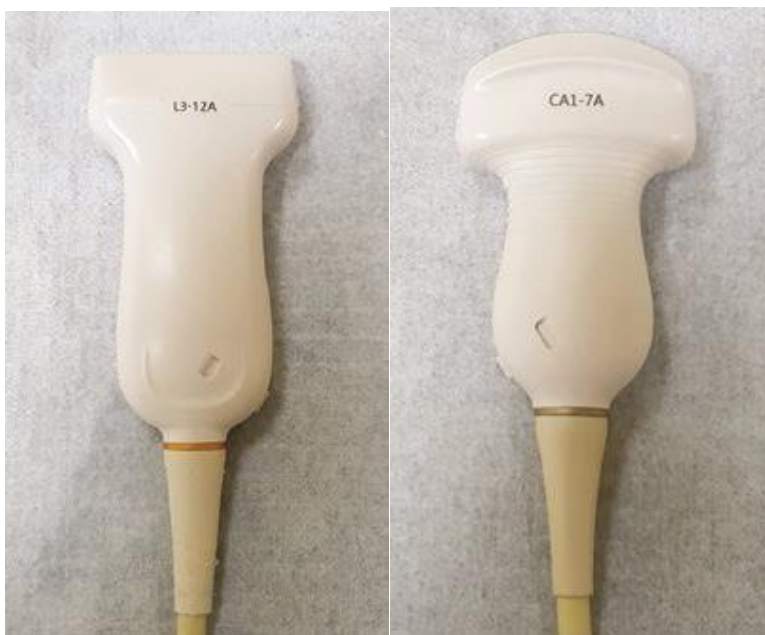
(Fig. 1): (a) Linear-array probe (5–12 MHz). (b) Convexarray probe (2–5 MHz) (5).
