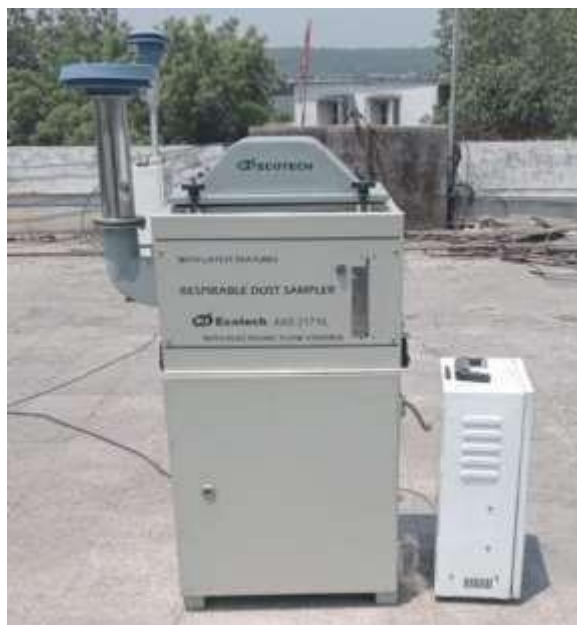
Fig. 2. Respirable dust sampler for PM 10 analysis
