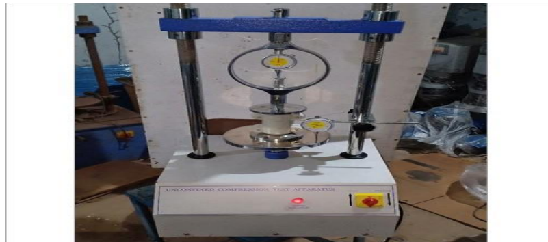
Fig 3.1 Unconfined Compressive Strength Test Apparatus
