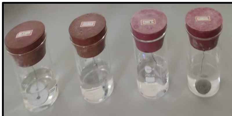
Figure 1: Immersion corrosion setup in HCl solution
