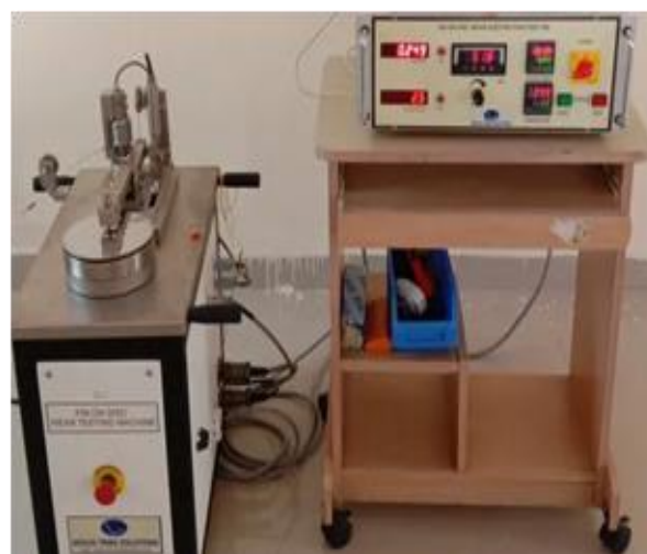
Figure 5: Ducom Pin-on-disc apparatus
