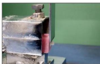
Fig 5. - Shear bond strength testing using universal testing machine
