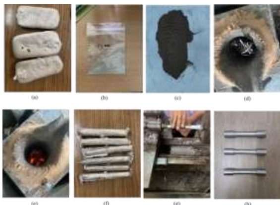
Fig 3. Preparation of samples (a) AA7068 ingots (b) Fly ash (c) Marble dust (d-e) Melting of composites (f) Cast specimens (g) Machining operation (h) Test specimens
