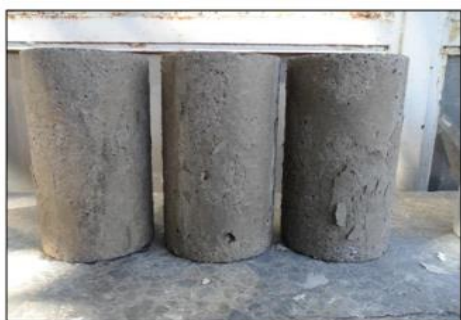
Figure 4.3. Surface deterioration of SCLWC specimens stored in magnesium sulphate solution
