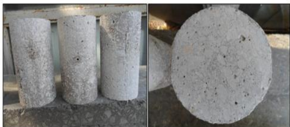
Figure 4.12. Surface deterioration of HSNWC specimens stored in sulphuric acid solution
