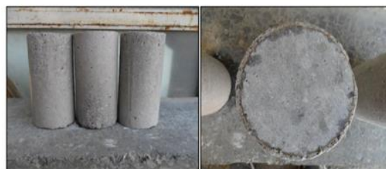
Figure 4.11. Surface deterioration of SCLWC specimens stored in sulphuric acid solution
