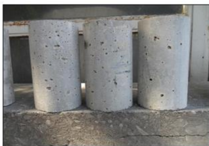
Figure 4.4. Surface deterioration of HSNWC specimens stored in magnesium sulphate solution
