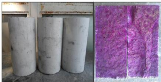
Figure 4.7. Surface deterioration of SCLWC specimens stored in sodium bicarbonate solution and interior of concrete tested by phenolphthalein
