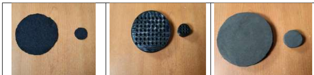
Fig2,3,4- Development samples of acoustic membrane,absorber plate,backing of 100mm and 30mm diameter restively.
