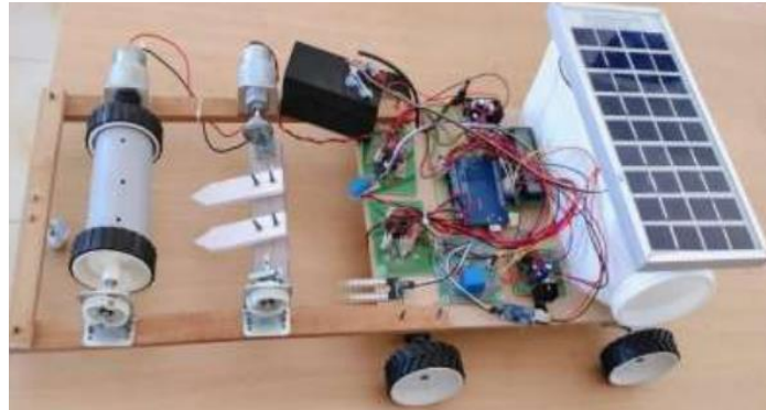
Figure.2: IoT based solar powered agriBot kit
