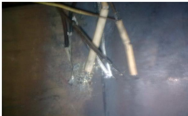
Fig 3 Mountings of nickel & nickel chromium thermocouples in weld coupon
