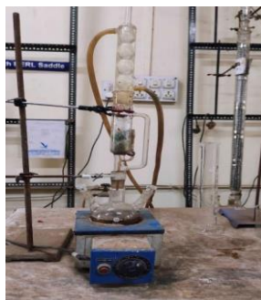
Figure 6: Extraction of Vinblastine (VBL) Using Soxhlet Extraction Method(at const. temp 800C)
