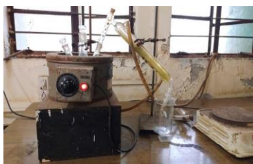
Figure 7: Simple Distillation to Separate the Sample From Solvent (at temp 700C)
