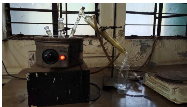
Figure 5: Simple Distillation Setup
