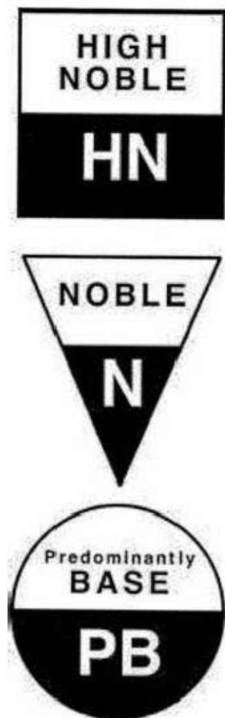
Fig.1 Symbols adopted by the ADA for its three major classifications of alloys based on composition
