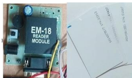
Fig. 3: RFID reader and RFID tag
