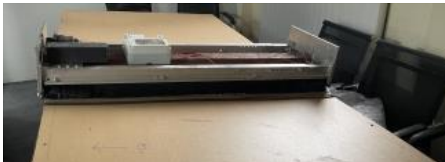
Fig. 4. Actual prototype for PV cleaner on the test bed
